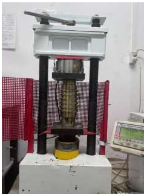
Figure 5 – The process of forming a sample on a hydraulic press
