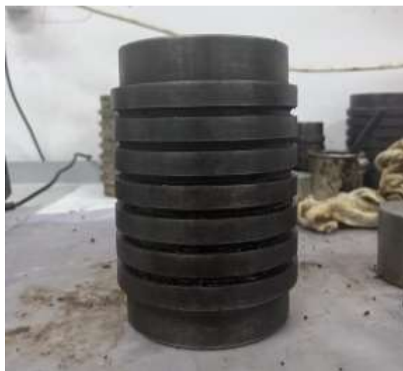
Figure 4 – Sample preparation mold
