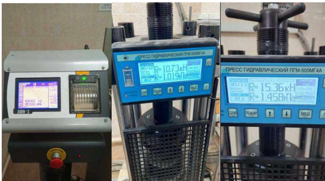
Figure 2 – Laboratory compression testing of concrete specimens
