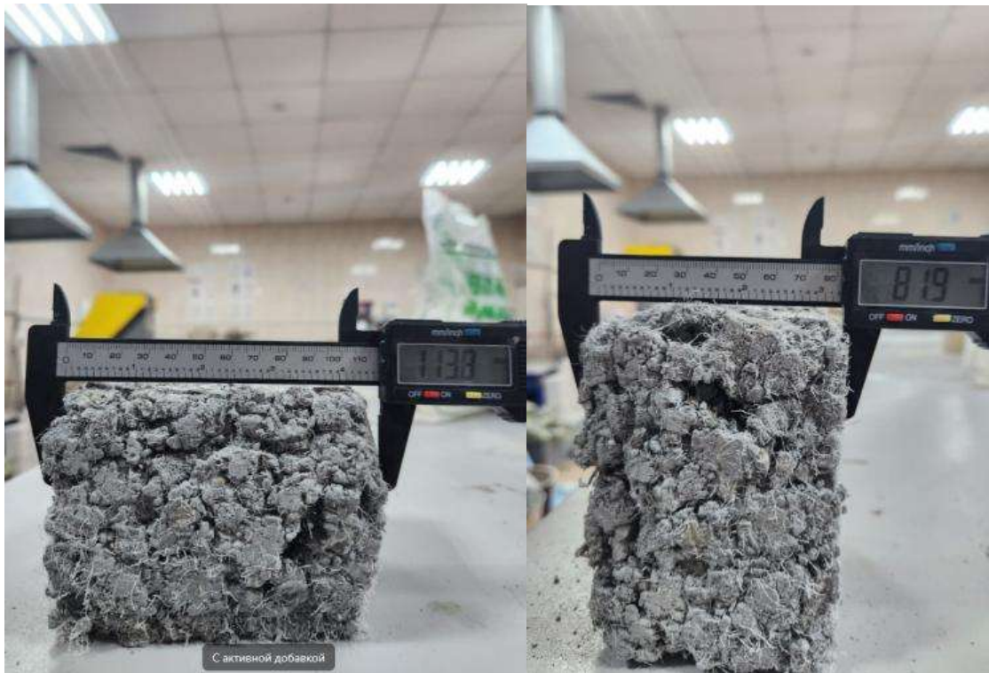
Figure 3 – Geometric indices of tested specimens of noise insulating concrete (NIC) after compression testing
