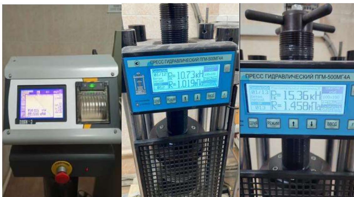
Figure 2 – Laboratory compression testing of concrete specimens
